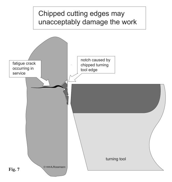
Chipped tools may be the death of high-cost components. A buried tool fragment may become a stress raiser that starts a fatigue crack in subsequent service. Often, close dimensional tolerances will bar repair. Tool failure, therefore,
