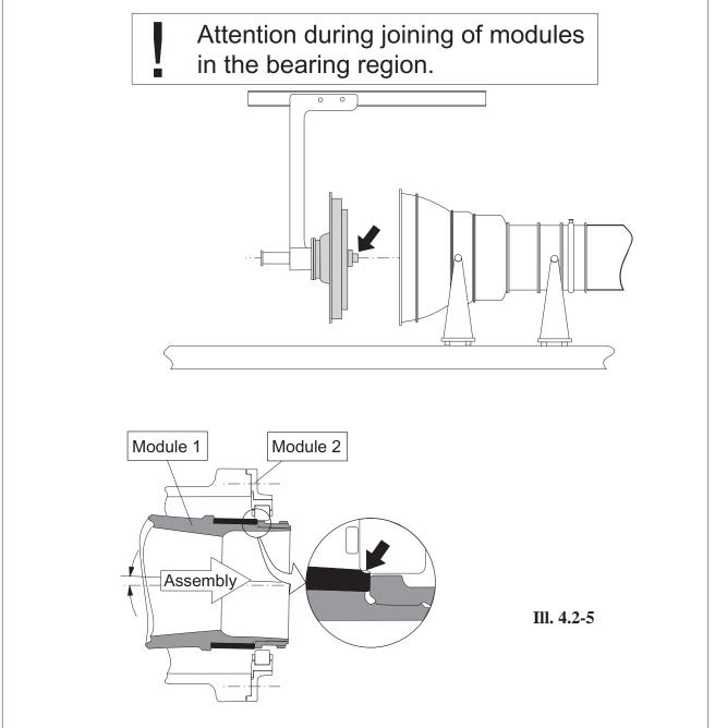
Ill. 4.2-5 (example 4.2-6): In the context of assembly work during inspection and overhaul, the situation arises that modules in the area of the bearing are joined. Here the joints (arrow in Fig. above) may sometimes be insufficiently visible. If it has to do with the difficulty to move masses, there is the possibility that the bearing, e.g. through the edge of the rolling body is
