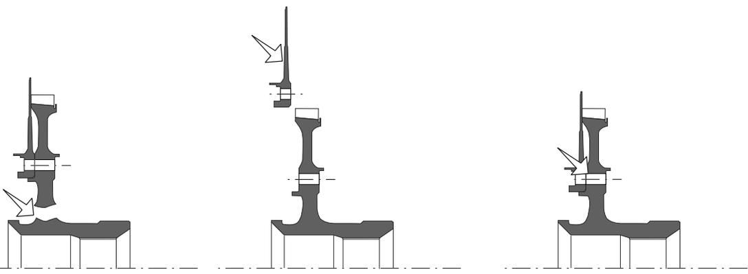
Fracture in the transition radius (operation fracture which could not be reproduced in a cyclical spin test).
