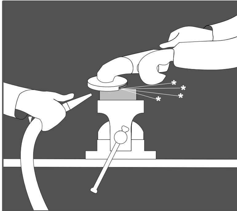
“**Damage reproduction**“ is a controlled process under defined test conditions which attempts to recreate damage that occurred during operation. A reproduction can only be regarded as successful if the damage has been simulated so that it is **identical to the original damage in both the micro and macro areas**. This is an extremely difficult task since damage is usually influenced by several different factors that act simultaneously.
