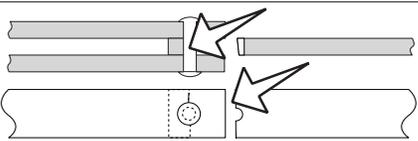
Failure due to low dynamic loads and friction damage (fretting)
