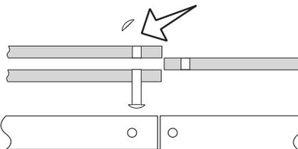
Dynamic fatigue fracture in the rivet head
