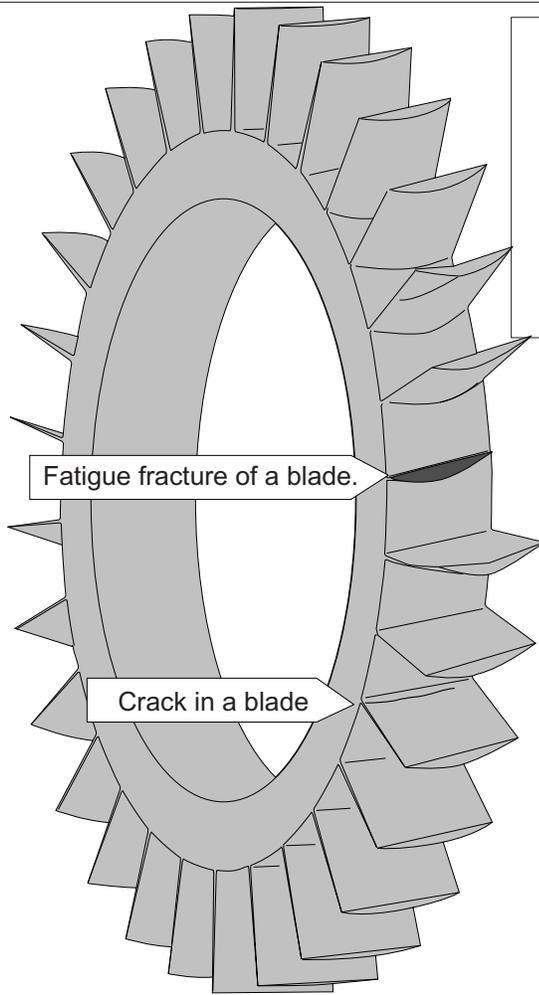
Possible causes for blade fracture and blade crack.
